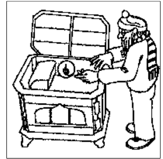
Always perform the "Match Test" before lighting your stove. If you light a match and hold it in front of the flue exit, the flame will be pulled into the flue collar if there is enough draft to light the stove.
